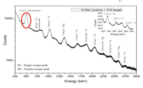
Typical spectrum measured for 30 nA current, with the rate of about 340 kHz and 120 s measuring time in Legnaro, 20x15 mm CeBr<sub>3</sub>, MPPC, TIA, MTCD
