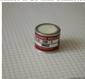
Fig. 1. Ø20×20 mm CeBr 3 scintillator, encapsulated in aluminium container with quartz window. The outer size of the container is 28 mm diameter and 24 mm height.
